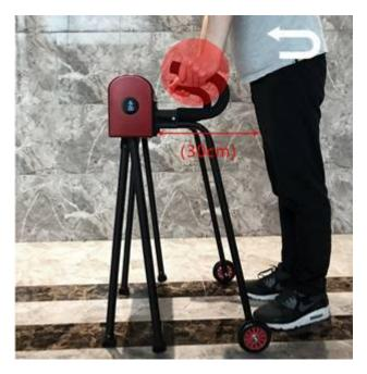
2) Push the robot horizontally with both hands, and the robot starts to step forward. The step speed matches the user apos; s hand pushing speed. The faster the push, the faster the step.
