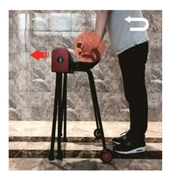
3) After waiting for the robot leg to land, the user moves forward one step, and the current operation is completed. Users need to gradually master the movement rhythm and follow the robot to move forward. Slowly cooperate with the robot to achieve the best use of the step valve.
